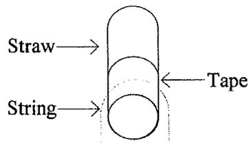
Figure 1: Wrap string around straw and secure with tape
